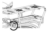
2. Slide the battery along the battery rail as far as possible into the battery holder.
